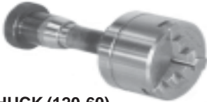
3-JAW CHUCK (120-60) 1-3/8" maximum opening with straight jaws 3-3/8" maximum opening with step jaws 3/4" thru hole With 5C adapter shank Hardened and ground tool steel
